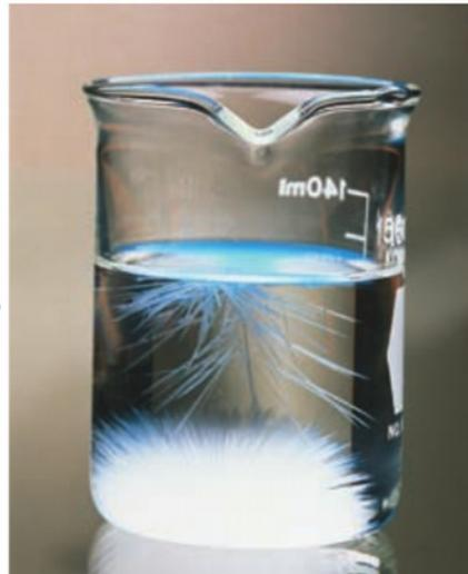
2 Excess sodium acetate crystallizes from solution
