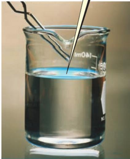
1 Seed crystal of sodium acetate added to supersaturated solution
